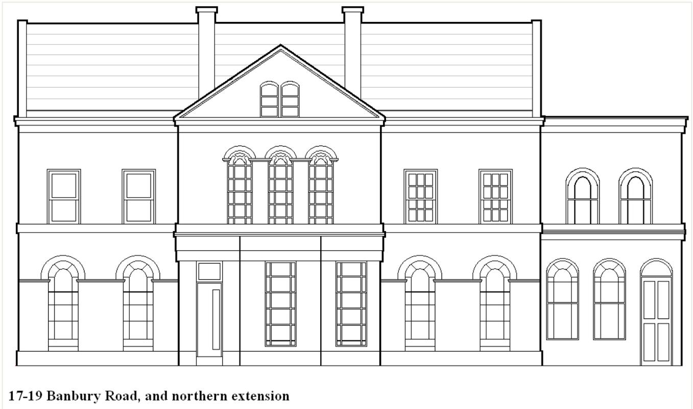
**Figure 3. Line drawing of eastern elevation of 17-19 Banbury Road and its northern extension. Note that there are now lightwells and railings in front of 15 and 19.**
